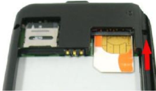
Install the first SIM card
